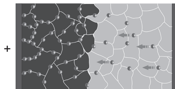
Figure 7. Schematic diagram of the influence of iodide ion migration on the PL intensity under an external electric field. The electric field drives the ions, leading to the accumulation of these ions which enhance the nonradiative recombination in these individual grains. These grain boundaries serve as the main pathways for the ionic migration.
