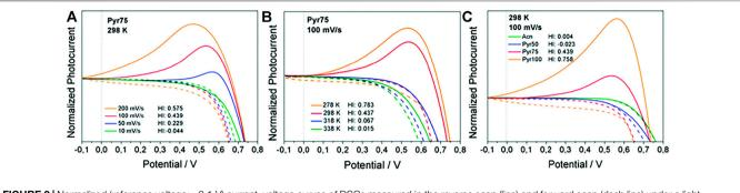
FIGURE 2 | Normalized (reference voltage: -0.1 V) current-voltage curves of DSCs measured in the reverse scan (line) and forward scan (dash line) under a light intensity of 10 mW cm<sup>-2</sup> using a green LED. The influence of hysteresis-determining factors is specifically shown: (A) scan rate, (B) temperature, and (C) electrolyte solvent. Reproduced from (Contreras et al., 2016).
