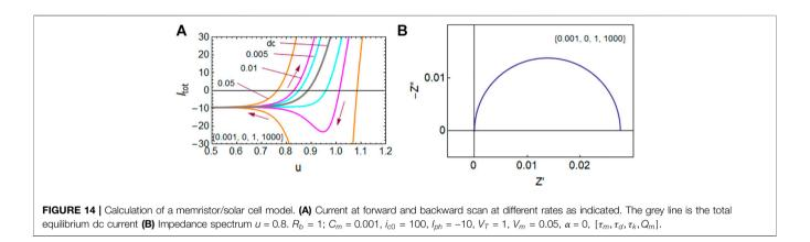
**Eq. 1** describes the components of  $I_{tot}$ : the photocurrent  $I_{ph}$ , the injection current  $i_{c0}f$ , a small ohmic current of constant resistance  $R_b$ , a capacitive charging of the interfaces with capacitance  $C_m$ , and a voltage-dependent capacitance correlated to f with a maximum surface charging  $Q_m$ .
