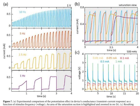
function of stimulus frequency (voltage). An area of the saturation section is highlighted and zoomed in on (b). (c) Resulting transient voltages in response to a train of rectangular current pulses of variable height, from 10  $\mu$ A to 1 mA, and 500 mHz, evidencing a clear static behavior in contrast of the dynamic effects obtained under voltage excitation.
