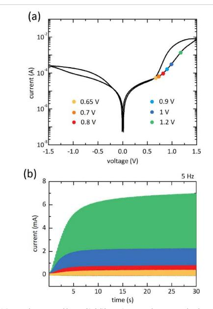
**Figure 3.** (a) Current–voltage response of the perovskite halide memristor measured at a scan rate value of 100 mV s<sup>-1</sup>, with consecutively increased voltage steps (5 mV) that induce gradual setting and resetting mechanisms. (b) Transient currents in response to a train of rectangular pulses of some of the indicated voltage in (a)—from 0.65 to 1.2 V—and 5 Hz, demonstrating the long-term potentiation of the device's conductance.
