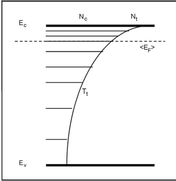
**Fig. 1.** Schematic energy diagram of the multiple-trapping transport picture. The horizontal scale indicates the density of traps in the band-gap. Representative model quantities are indicated: effective density of transport states  $N_c$ , band-gap energy  $E_c-E_v$ , effective density of trap states  $N_t$ , characteristic trap temperature  $T_t$  (determining the shape of the exponential tail) and the average Fermi level ( $E_F$ ).
