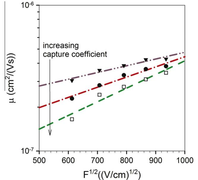
Fig. 4. Model representation of mobility versus  $F^{1/2}$  by the IS technique for different capture coefficients  $c = 7 \times 10^{-13}$ ,  $4 \times 10^{-12}$ ,  $9 \times 10^{-12} \text{ cm}^3/\text{s}$ , from top to bottom. Mobility fittings are ranged as:  $1.6 \times 10^{-7} \text{ cm}^2/(\text{Vs}) > \mu_0 > 4.8 \times 10^{-8} \text{ cm}^2/(\text{Vs})$  and  $1.1 \times 10^{-3} (\text{cm/V})^{1/2} < \gamma < 2.2 \times 10^{-3} (\text{cm/V})^{1/2}$ .
