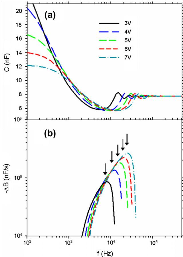
Fig. 3. Model representations at voltages ranging from 3 V to 7 V. (a) capacitance spectra and (b) negative differential susceptance extracted from the upper panel.
