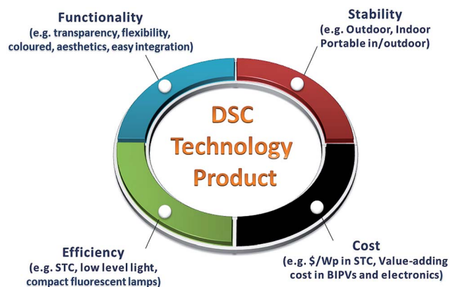
Fig. 17 Scheme representing inter-relationships between the three parameters (power conversion efficiency, stability and cost) that must be considered together with functionality for the successful industrial product development of dye-solar cell modules. Different applications and markets lead to different mixes of requirements and thus different DSM technological developments ( e.g. , glass, flexible, material combinations, device architectures, etc. ).
