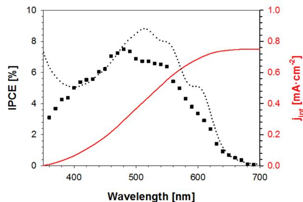
**Figure 4.** IPCE spectrum (squared dots) and integrated current (red solid line) of a representative ITO/x-PEDOT/BHJ/ $\text{TiO}_x$ /Pt (50 nm) device. The absorbance spectrum of the device is also shown (dotted line).
