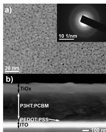
**Figure 2.** (a) Transmission electron microscopy (TEM) micrographs of a thin layer of  $\text{TiO}_x$  nanoparticles. Inset: Diffraction pattern showing that the material is highly amorphous. (b) Cross-section scanning electron microscopy (SEM) image of the most stable device configuration.
