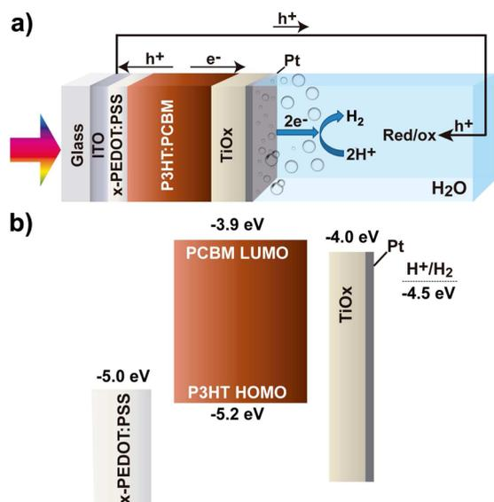
**Figure 1.** (a) Device architecture of the optimized organic photoelectrochemical cell (OPEC) developed in the present study showing the electronic processes taking place during device operation. (b) Energy diagram of the device with literature values measured under vacuum conditions.
